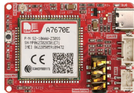
Crowtail 4G SIM A7670E Module GPS Breakout Board support GPS/GLONASS/BDS
