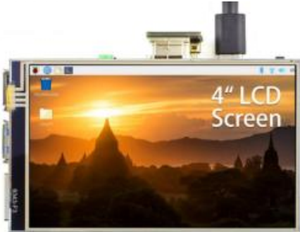
RR040I 4 inch HD 800x480 Resolution IPS TFT Touch Screen Display for Raspberry Pi
